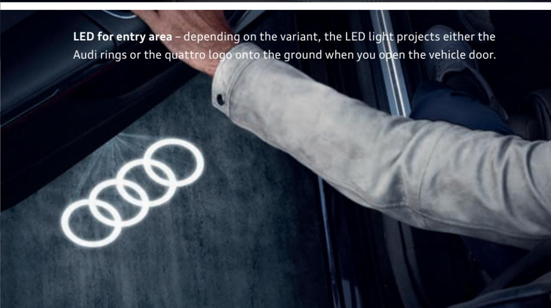
**LED for entry area** – depending on the variant, the LED light projects either the Audi rings or the quattro logo onto the ground when you open the vehicle door.
