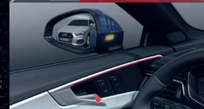
**Exit warning<sup>1</sup>** – detects vehicles and cyclists approaching from the rear and in critical situations warns occupants before they open the doors
