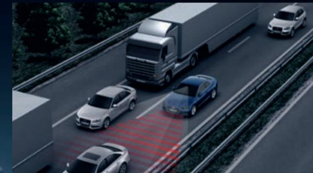
**Audi pre sense city<sup>1</sup>** – can help to prevent imminent collisions with vehicles and pedestrians at vehicle speeds of up to approximately 85 km/h by giving warning signals and applying the brakes
