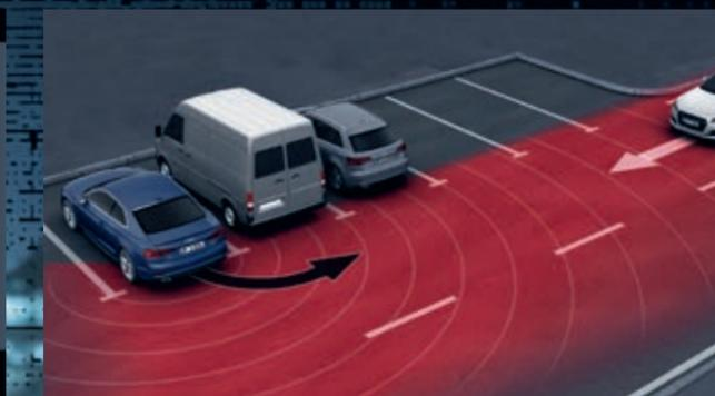
**Cross traffic assist rear<sup>1</sup>** – shows approaching vehicles in the MMI display when reversing out of bay parking spaces and can help to avoid critical situations by issuing a warning tone and briefly tapping the brakes
