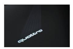
The entry LED projects the quattro lettering onto the ground when the front doors are opened.
