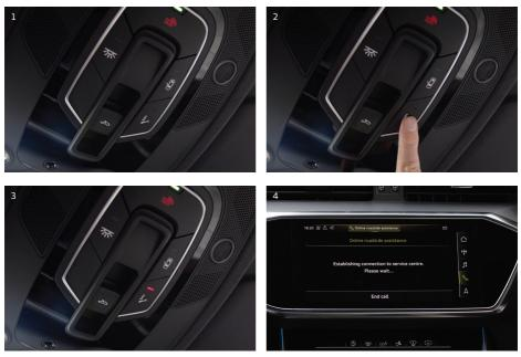
\*In the event of an accident, the vehicle occupants can place a call for assistance by pressing the Online Roadside Assistance button in the roof module, or in case of emergency press the red SOS button. Please refer to the Owner's manual for further details on using these functions.
