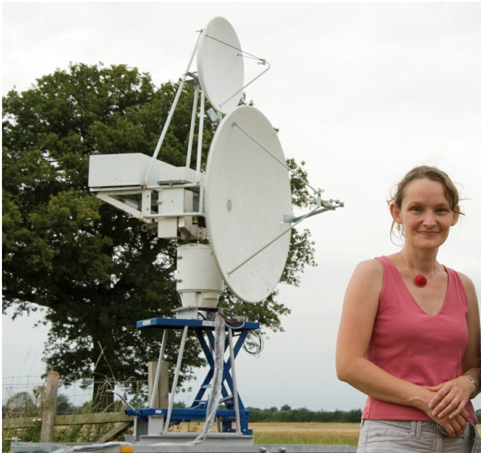
Juliet Osborne, a pioneer in the application of modern radar-technology to behavioural research on honeybees, and the associated apparatus (lower disc – transmitter; upper disc receiver). (Photo: A. Martin)
