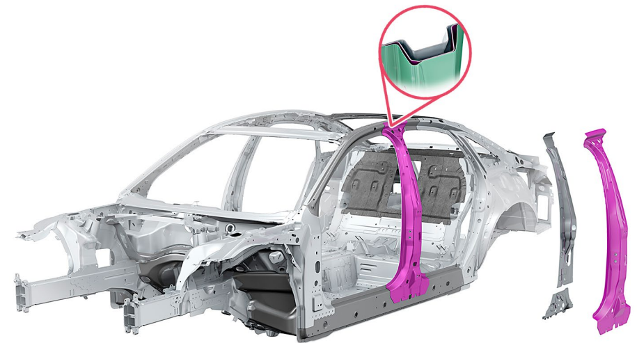
B-pillar with multi-shell structure
