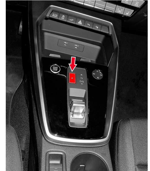
Vehicles with an automatic gearbox without a selector lever: press the “P” button
