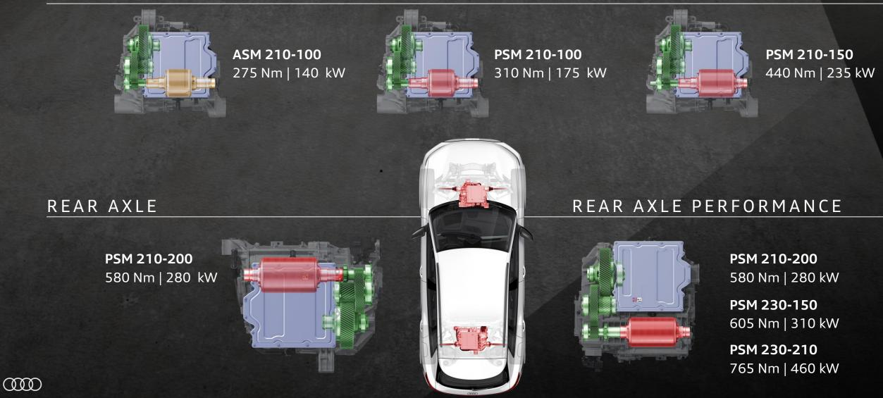
Compared to 1st generation BEV – PPE drivetrains offer sizeable performance improvements and cost reduction
