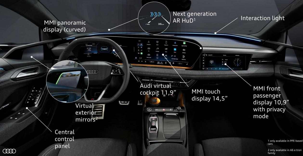
The new augmented reality head up display offers increased field of view as well as improved imaging and expanded functionality
