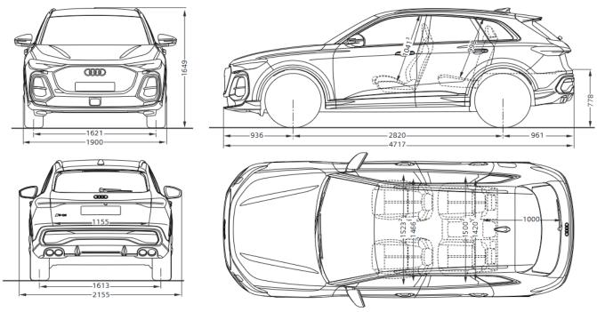
$^{\rm 5} All$  measurements are in millimetres. S line model shown.
